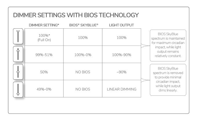
• Very important: Once a maximum lumen output has been set, dimming up from the 'learned' maximum will increase the light fixtures' lumen output but it will not increase the m:p ratio. Once a maximum lumen output is set, the m:p ratio is essentially capped or set to be maximized for that lumen output, therefore the m:p ratio cannot be increased until the system 'learns' a new higher setpoint.
